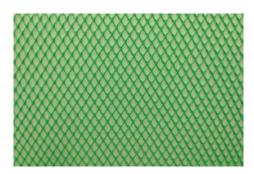
Airtechs' Greenflow 75 is a high performance, low profile resin distribution medium designed to promote resin flow during the vacuum infusion process. The tight, low profile crisscross pattern of the infusion mesh distributes a controlled, predictable flow of resin throughout the laminate efficiently and with little waste. The resin will flow slightly slower compared to the red infusion mesh.
